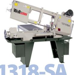
Semi-Automatic-We added the efficiency of a PLC controller to the strength and precision of our popular model 1318. The model 1318-SA Semi-Automatic eliminates the time consuming operations of a manual saw so that you get more safety, fewer mistakes, and increased output. The model 1318-SA offers all the features of our model 1318 plus;
