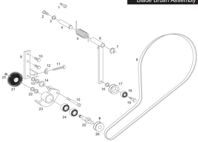
Note: Adjust thumb screw (11) so that the brush makes light contact with the blade. This avoids dulling the blade and prevents premature brush wear.
