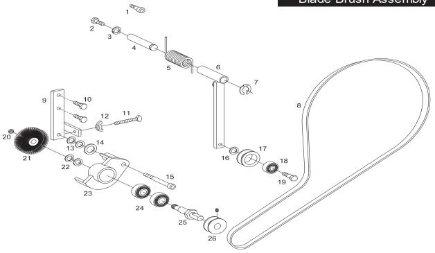
Note: Adjust thumb screw (11) so that the brush makes light contact with the blade. This avoids dulling the blade and prevents premature brush wear.
